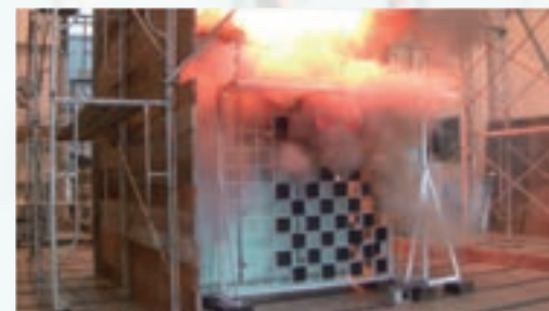
JSB-5 internal arc test (31.5 kA 1 sec)
