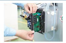
Circuit boards can be replaced individually in the event of a system malfunction, ensuring quick recovery and minimal running costs
