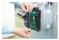
Circuit boards can be replaced individually in the event of a system malfunction, ensuring quick recovery and minimal running costs
